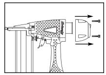
Figure 6. Removing the exhaust cap.
